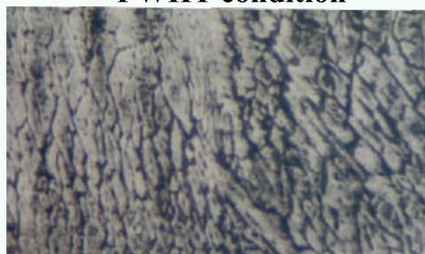
Optical micrographs of welded joints in as-welded & PWHT conditions
